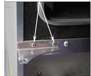
17. Fit screws removed at Item 14 above to where hinges were fitted.
